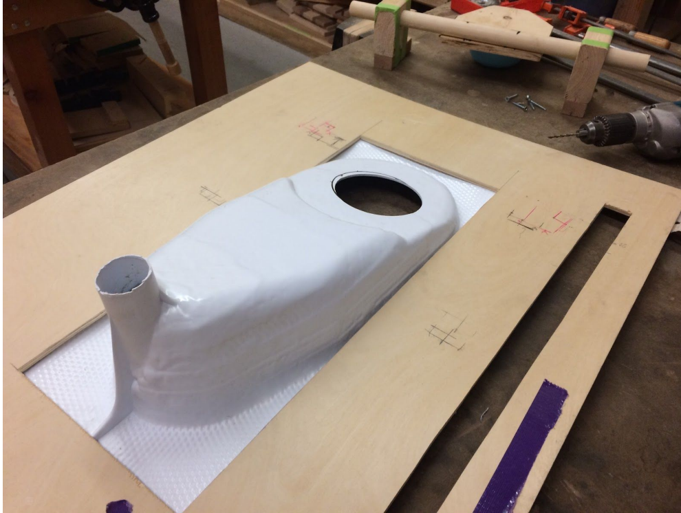
Figure 11: The ledge at the back of the squat pan prevents the flap from sitting flush with the feces hole.
