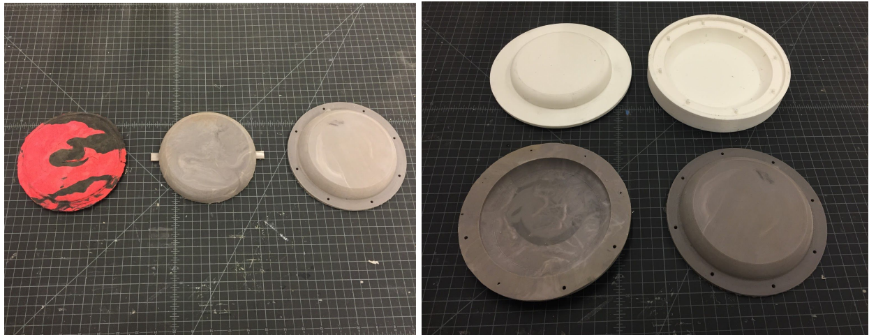
Figure 8: Prototyping seal shape (left), final seal and 3D printed mold (right).
