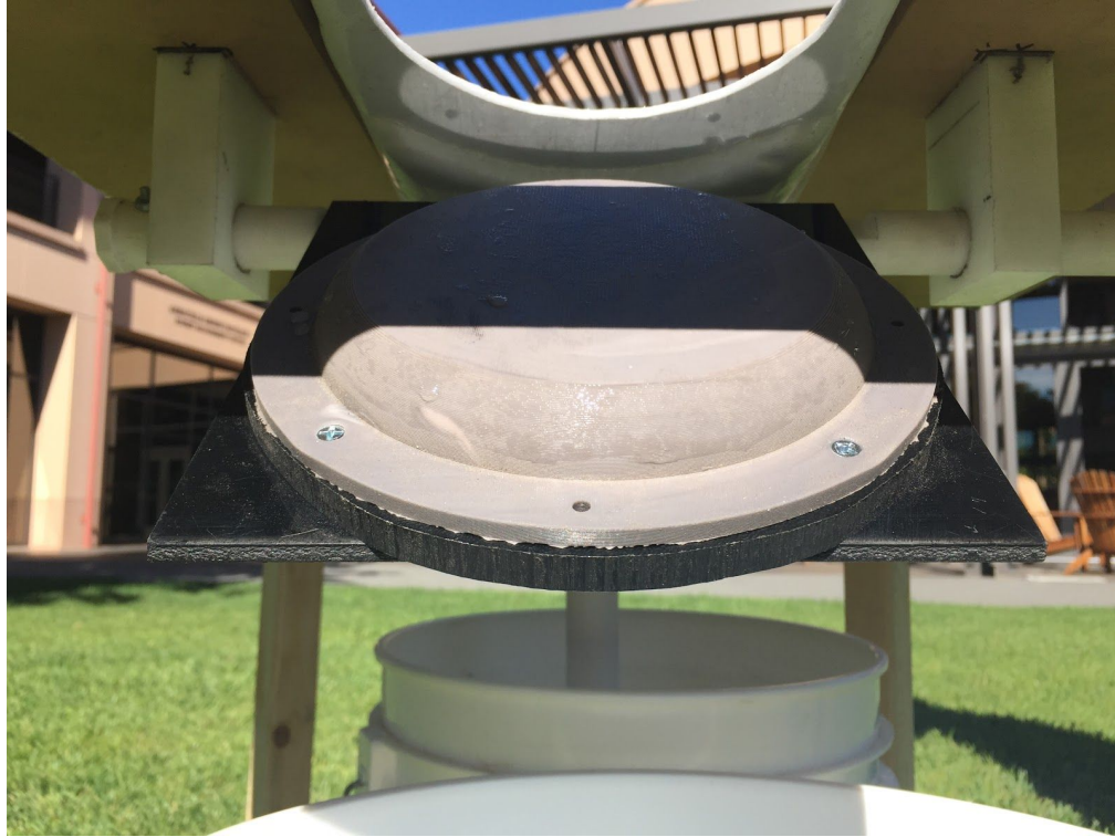
Figure 10: The seal works very well, as evident by the dry area below where the plug interfaces with the edge of the feces hole.
